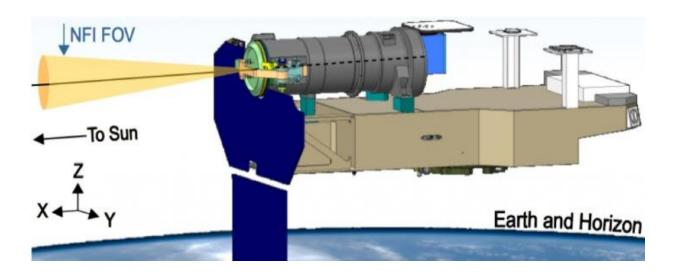
US Naval Research Laboratory's Narrow Field Imager shown on one of the four PUNCH micro-satellites. PUNCH will provide imaging of the solar wind from low Earth orbit. Work was funded by NASA. Credit: PUNCH Team/Southwest Research Institute
