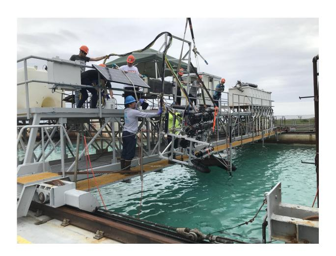
A team of New Jersey Institute of Technology (NJIT) researchers is conducting oil dispersion experiments at the 600-ft.-long salt water wave tank at the US Department of the Interior's Ohmsett facility on the Jersey Shore. Credit: NJIT
