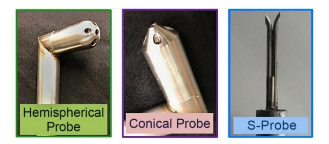
NIST designed two new pitot probes (left and center), one whose sensing surface is cone-shaped and the other whose surface is hemispherical. The probes have five holes, or ports. Comparing pressure readings obtained in each of the five ports allows technicians to calculate the flow rate. An older type of pitot tube, called an S-probe (right), has two ports that face in opposite directions. Credit: NIST
