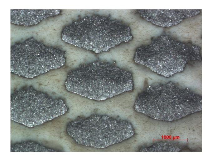
Optical image of material surface after erosion testing with speed of 30 m/s and impact angle of 30 degrees. Credit: Rahul Kumar
