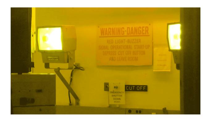
The long-term radiation dose tests at the Radiation Effects Facility take place in a small room walled by four feet of concrete. Each part of every NASA instrument destined for spaceflight goes through radiation testing to ensure it can survive in space. Credit: NASA's Goddard Space Flight Center/Genna Duberstein
