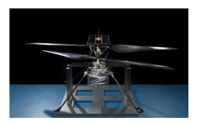
This image of the flight model of NASA's Mars Helicopter was taken on Feb. 14, 2019, in a cleanroom at NASA's Jet Propulsion Laboratory in Pasadena, California. The aluminum base plate, side posts, and crossbeam around the helicopter protect the helicopter's landing legs and the attachment points that will hold it to the belly of the Mars 2020 rover. Credit: NASA/JPL-Caltech
