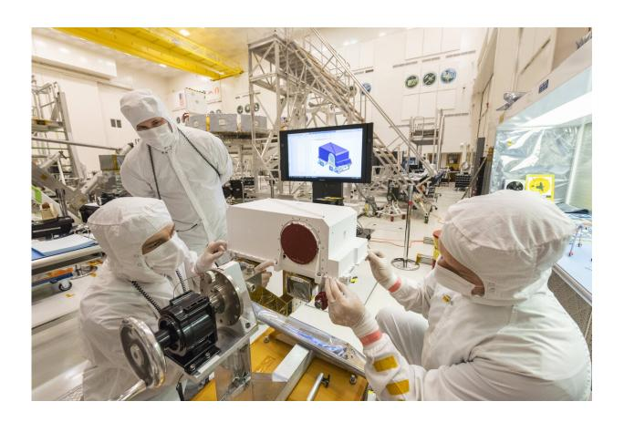
In this picture - taken on May 23, 2019, in the Spacecraft Assembly Facility's High Bay 1 clean room at the Jet Propulsion Laboratory in Pasadena, California - engineers re-install the cover to the remote sensing mast (RSM) head after integration of two Mastcam-Z high-definition cameras that will go on the Mars 2020 rover. Credit: NASA/JPL-Caltech
