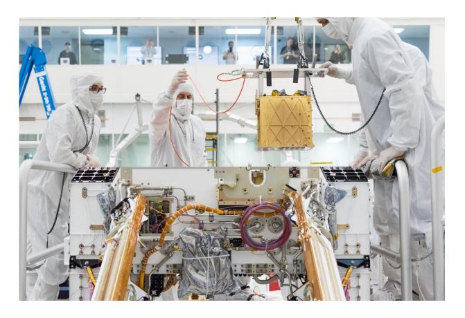
Members of NASA's Mars 2020 project install the Mars Oxygen In-Situ Resource Utilization Experiment (MOXIE) into the chassis of NASA's next Mars rover. MOXIE will demonstrate a way that future explorers might produce oxygen from the Martian atmosphere for propellant and for breathing. Credit: NASA/JPL-Caltech
