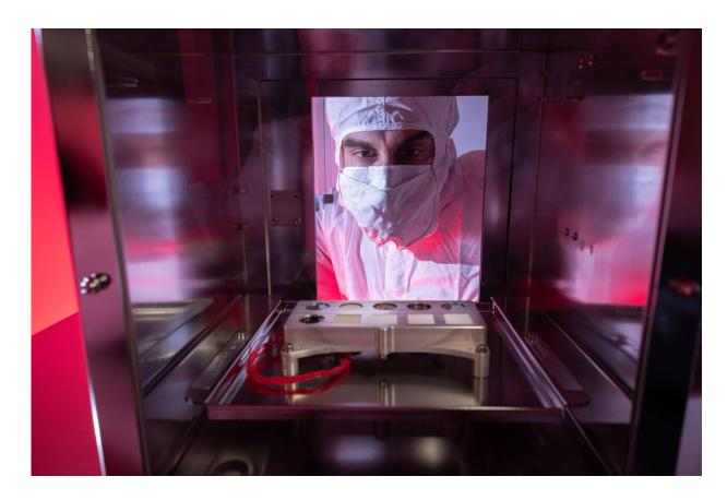
This calibration target for Mars 2020's SHERLOC instrument includes five samples of spacesuit material, the first to ever be flown to the Red Planet. By studying how these samples degrade in the Martian environment, engineers can develop better spacesuits. Credit: NASA
