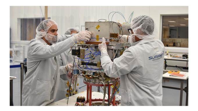
Technicians integrate NASA's Deep Space Atomic Clock into the Orbital Test Bed Earth-orbiting satellite, which will launch on a SpaceX Falcon Heavy rocket, on June 22, 2019. Credit: General Atomics
