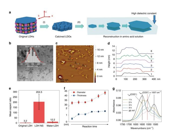
High aspect ratio LDH nanosheets. a Schematic showing (I) calcination (interlayer water and anions are removed by calcination) and (II) reconstruction process and the preferential growth inhibition in a high dielectric constant
