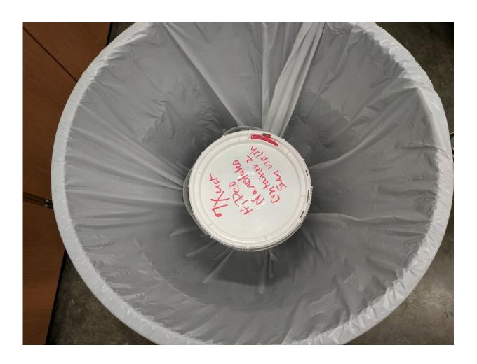
A plastic bucket and a plastic bag contain a 5-gallon supply of carbon nanotubes in a lab at Rice University, the beginning of the process to safely transfer the nanotubes for experimental use. The Rice lab published its technique in *SN Applied Sciences*. Credit: Barron Research Group/Rice University
