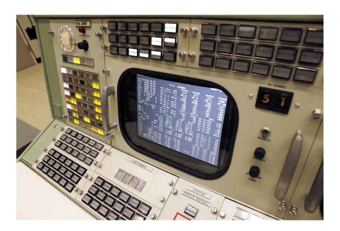
A screen displays simulated telemetry data on the the console for the Booster Systems Engineer, the first position on the first row known as "The Trench", inside the Apollo mission control room as it is restored to replicate the Apollo mission era for the 50th anniversary of the Apollo moon landing at the NASA Johnson Space Center Monday, June 17, 2019, in Houston. (AP Photo/Michael Wyke)
