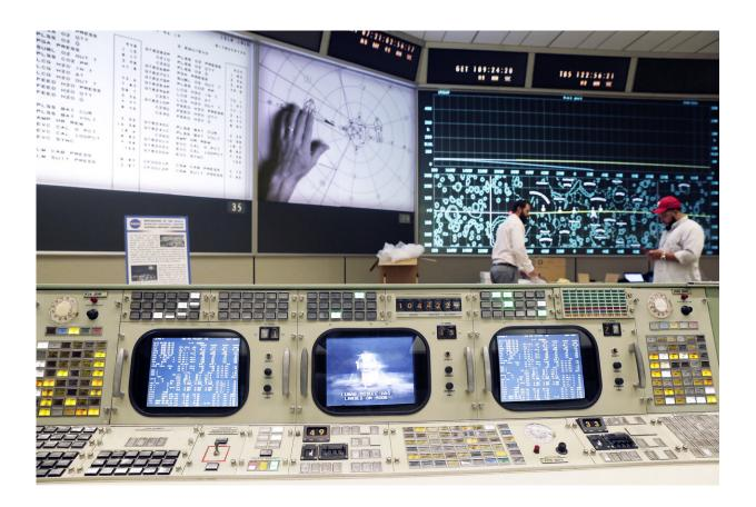
The console for Booster Systems Engineer, the first position on the first row known as "The Trench," has an overview of the Display and Projection screens
