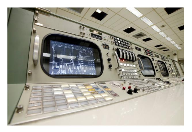
A rotary dial and other controls are shown on the console for the Instrumentation and Communications Officer, the 11th position on the third row inside the mission control room being restored to the Apollo mission era for the 50th anniversary of the Apollo moon landing at the NASA Johnson Space Center Monday, June 17, 2019, in Houston. (AP Photo/Michael Wyke)
