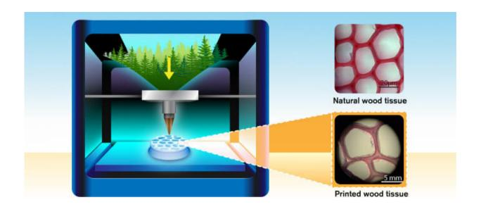
Mimicking the natural cellular architecture of wood. The printed version is at a larger scale for ease of handling and display, but the researchers are able to print at any scale. Credit: Yen Strandqvist/Chalmers University of Technology
