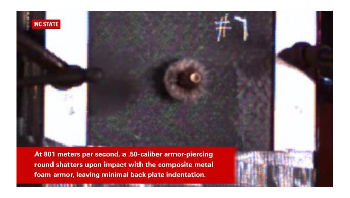
Researchers have demonstrated that vehicle armor using composite metal foam (CMF) can stop ball and armor-piercing .50 caliber rounds as well as conventional steel armor, even though it weighs less than half as much. The finding means that vehicle designers will be able to develop lighter military vehicles without sacrificing safety, or can improve protection without making vehicles heavier.
