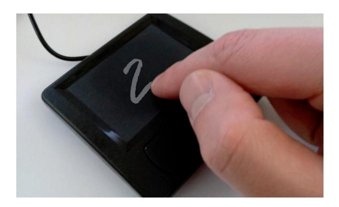
AIfES demonstrator for handwriting recognition. Numbers written by hand on the PS/2 touchpad are identified and output by the microcontroller. Credit: Fraunhofer-Gesellschaft
