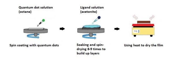
The team developed a new thermoelectric material by spin coating a liquid solution of nanomaterials and then spin coating a series of thin layers of lead-sulphide quantum dots onto the surface. They dried the film using thermal annealing. Credit: WILEY-VCH Verlag GmbH & Co. KGaA, Weinheim
