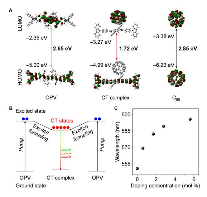
Theoretical investigation of the CT processes in light-harvesting systems. (A) Molecular orbital diagrams of OPV, C60, and CT complex calculated by density function theory. (B) Schematic of efficient exciton funneling for the formation, accumulation, and radiative deactivation of CT excitons in the C60@OPV light-harvesting systems. (C) Maximum emission wavelength of microcrystals versus C60 doping concentration. Credit: Science Advances, doi: 10.1126/sciadv.aaw2953
