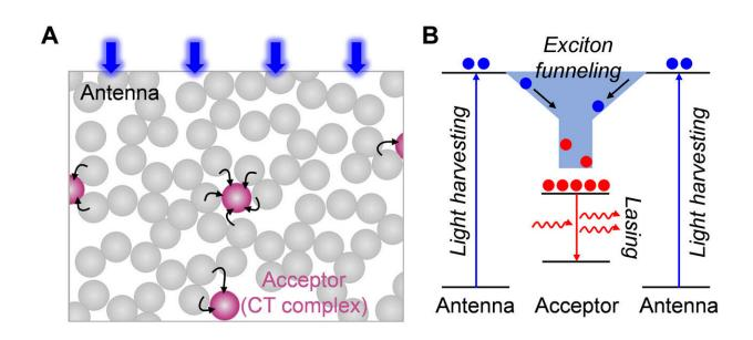
Illustration for exciton funneling in the light-harvesting systems. (A) Schematics of light harvesting, where the wide-bandgap hosts (gray spheres) act as antenna and locally formed CT complexes with narrow bandgap (pink spheres) act as acceptor. (B) Diagram for exciton funneling in light-harvesting systems. The black arrows represent the exciton transfer process. Credit: *Science Advances*, doi: 10.1126/sciadv.aaw2953
