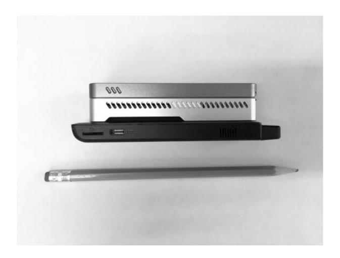
A 2016 SETG solution for portable single molecule DNA sequencing: nanopore MinION (top) device and Intel Compute Stick, controlled with a smartphone. Credit: C.E. Carr
