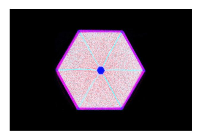
Cross-section of a nanowire featuring a gallium arsenide core, an indium aluminum arsenide shell, and an indium gallium arsenide capping layer (gallium is shaded blue, indium red and aluminum cyan). The image was produced by energy-dispersive X-ray spectroscopy. Credit: HZDR / R. Huebner
