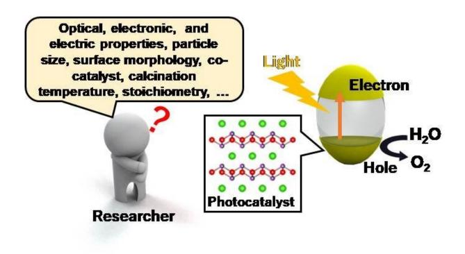
(Right) Schematic of photocatalytic reaction. (Left) Many factors that affect the photocatalytic performance. Credit: Osaka University
