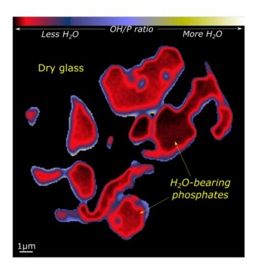
A NanoSIMS isotope ratio image showing water-bearing minerals (colors) in a sea of water-poor glass (black) in Apollo sample 10049. These were the last
