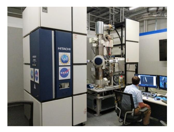
Tom Zega at the control panel of the 12-foot tall transmission electron microscope at the Kuiper Materials Imaging and Characterization Facility at the UA's Lunar and Planetary Lab. The instrument allows researchers to see individual atoms in extraterrestrial samples. Credit: Daniel Stolte/UANews
