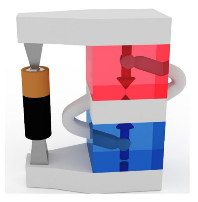
Interlayer coupling interaction. Two ferromagnetic layers (red, blue) antiparallel aligned (arrows indicate the direction from the south to the north pole) are forced by this electronic effect to 'twist' their magnetization (as indicated by the arms) adding a chirality (preferential rotation sense). Credit: Eindhoven University of Technology
