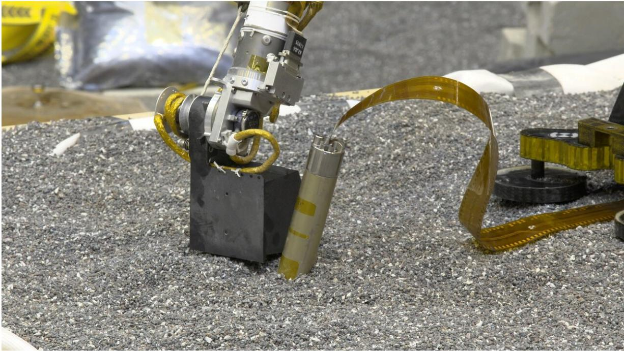
In a JPL lab, a replica of NASA InSight's robotic arm presses with its scoop on crushed garnet near a replica of the spacecraft's self-hammering "mole." Engineers believe pressing like this on Martian soil may help the mole dig by increasing friction of the surrounding soil. Credit: NASA/JPL-Caltech
