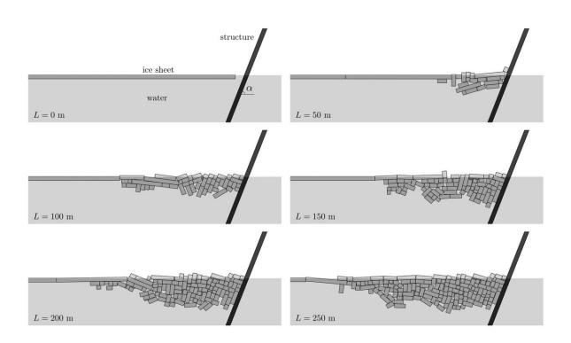
An example of numerical experiments on sea ice using computer simulations. An ice sheet collides with an inclined structure and fails into individual ice blocks, which form a rubble pile. This type of simulation helps in gaining detailed understanding of the mechanics of sea ice. Credit: Arttu Polojärvi/Aalto University
