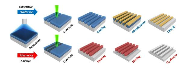
IL process flow. Water ice acts as a positive-tone lithography resist, and alkane ice demonstrates a negative-resist-like capability. Credit: Science China Press
