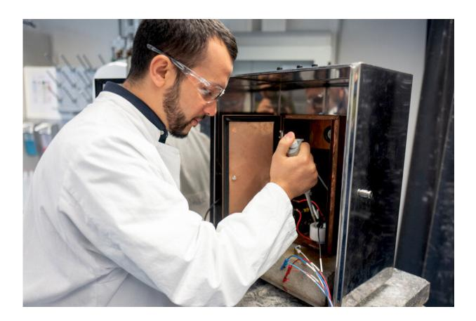
In this shielded cell, Abdelilah El Arrassi is testing the nanoparticles in electrochemical experiments. Credit: RUB, Kramer
