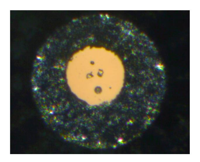
Hurlbutite crystals (centre) in the diamond anvil cell used for the high pressure experiments. The crystals are each about 0.01 millimetres in size. Credit: DESY, Anna Pakhomova
