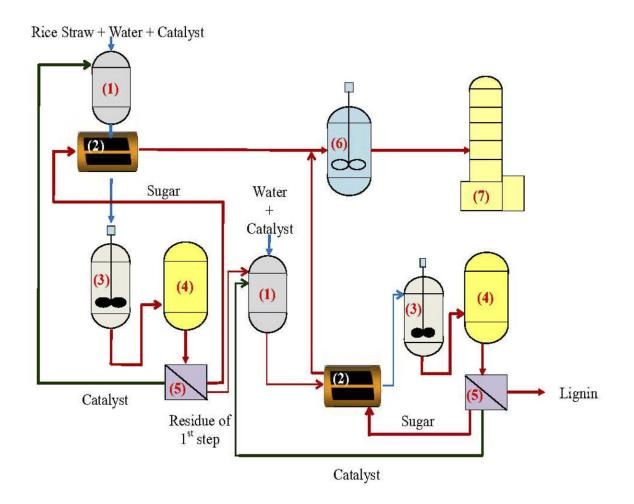
Researchers designed two-step process to break down rice straws into sugars for fuel. Credit: Figure adapted from *Ind. Eng. Chem. Res.* 2019 58 (14), 5686-5697. © 2019 American Chemical Society
