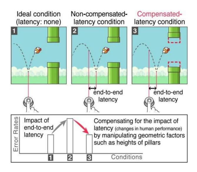
Figure 1. Overview of Geometric Compensation
