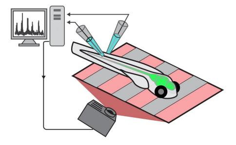
In a virtual reality tank, scientists could trick zebrafish into feeling like they weren't swimming, even though they were paddling hard. This image shows the experimental setup -- electrodes inserted into the fish larvae measured brain cells' behavior in the virtual reality tank. Credit: Ahrens Lab/Janelia Research Campus
