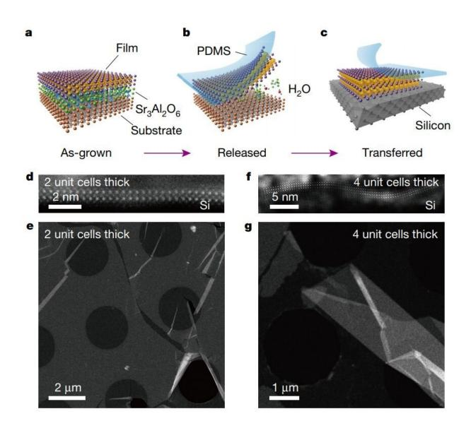
Growth and transfer of ultrathin freestanding SrTiO3 films. a, Schematic of a film with an SAO buffer layer. b, The sacrificial SAO layer is dissolved in water
