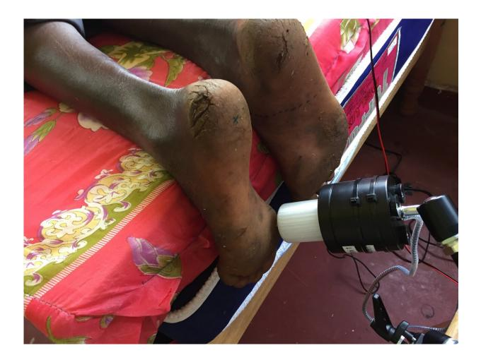
Custom-built device used to measure tactile sensitivity of foot at different frequencies. Credit: Daniel Lieberman
