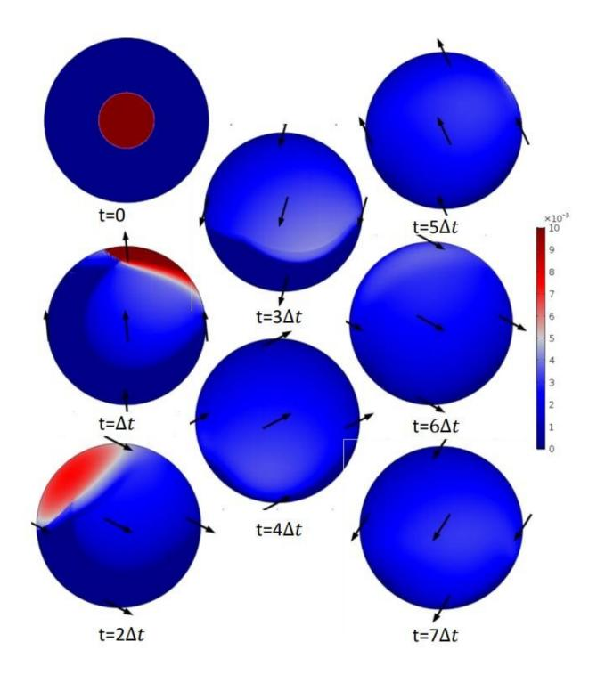
Contours of film thickness h(x, t) for the optimal harmonic kinematics minimizing U(tf), obtained with the Monte-Carlo method. Credit: arXiv:1901.06028 [physics.flu-dyn]
