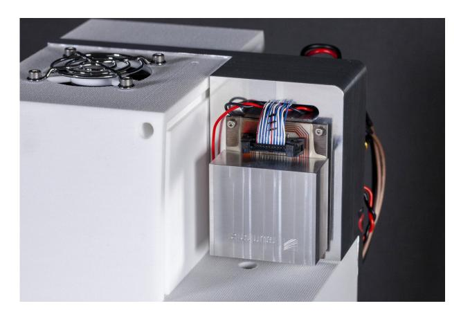
The core of the system is an extremely fast tunable quantum cascade laser with emission wavelengths in the mid-infrared range and high scan frequencies of up to 1 kHz. Credit: Fraunhofer Institute for Applied Solid State Physics IAF
