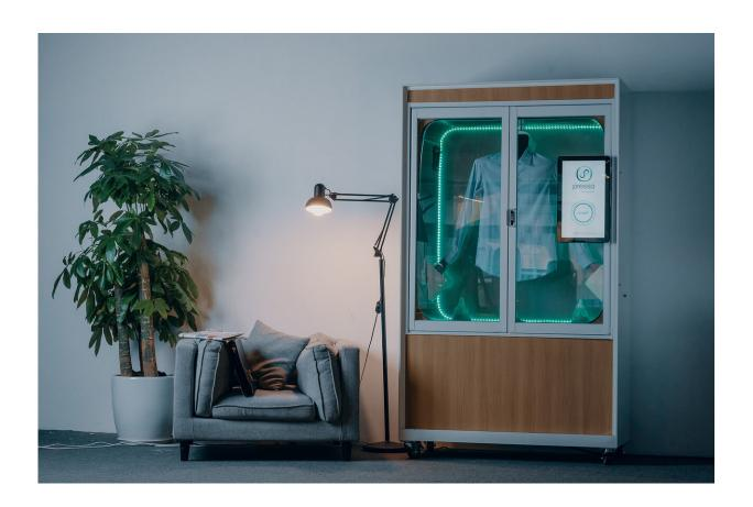
Two Purdue University graduates are developing a device called Presso, a kiosk garment cleaning device that takes only three to seven minutes to clean clothes through a combination of steam, a cleaning liquid and air drying. The kiosk is less expensive than conventional dry cleaning and also more environmentally friendly. Credit: Purdue University
