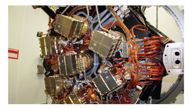
The second core component of the telescope is the X-ray camera system. At the focal point of each mirror system is a highly sensitive CCD detector that was specially developed for eROSITA in the semiconductor laboratory at the Max Planck Society. These detectors are a further development of existing X-ray CCD cameras. Credit: German Aerospace Center (DLR)
