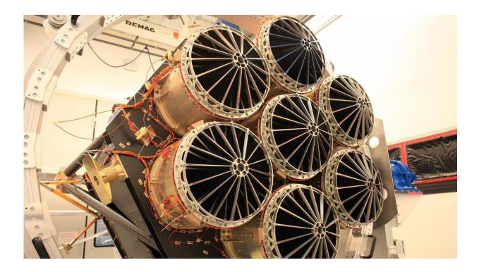
The first core component of the eROSITA space telescope consists of seven identical mirror modules aligned in parallel. Each has a diameter of 36 centimetres and consists of 54 nested mirror shells whose surface is composed of a paraboloid and a hyperboloid (Wolter I optics). They collect high-energy photons and focus them onto the X-ray cameras. Credit: German Aerospace Center (DLR)
