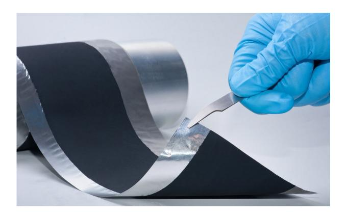
This is what the electrodes coated with the new dry transfer coating technology look like. Fraunhofer IWS process enables battery electrodes to be produced on a pilot scale without using toxic solvents. Credit: Fraunhofer-Gesellschaft
