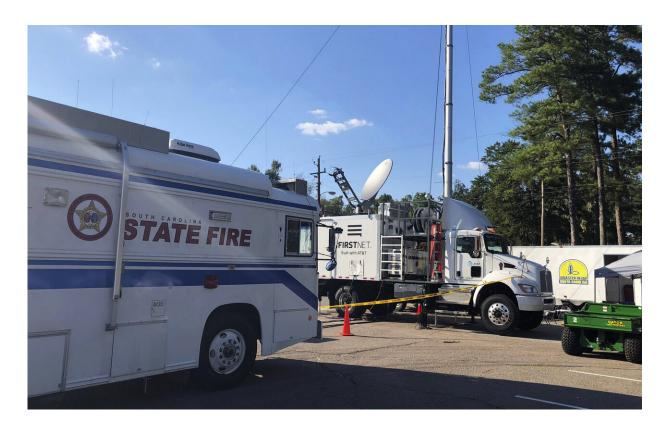
This Sept. 19, 2018, photo provided by AT&T shows equipment, center, that turns a satellite signal into an LTE cell tower that was used during Hurricane Florence in Marion, South Carolina. The equipment is a supplementary part of FirstNet, a new national wireless network dedicated for first responders. A major earthquake that rocked Alaska proved to be a trial run in the state's largest city for a new national wireless network dedicated to first responders. (AT&T via AP)
