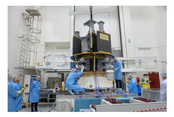
SSMS vibration testing. Credit: ESA - M. Pedoussaut
