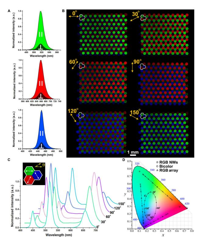
Polarizer tunable color multiplexing. (A) Polarized PL spectra of the printed nanocomposites incorporating CsPbBr3 (green), CsPb(Br0.2I0.8)3 (red), and CsPb(Br0.2Cl0.8)3 (blue) nanowires, taken with a pair of two linear polarizers
