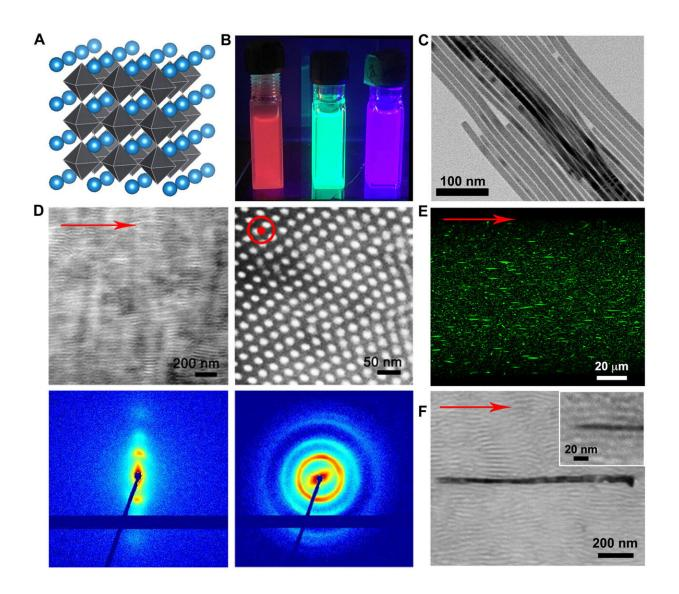
Perovskite nanowire–block copolymer supramolecular nanocomposites. (A) Schematic diagram of the perovskite crystal structure. (B) PL of CsPbX3 (X = I, Br, and Cl) perovskite nanowires in toluene solution. Halide composition
