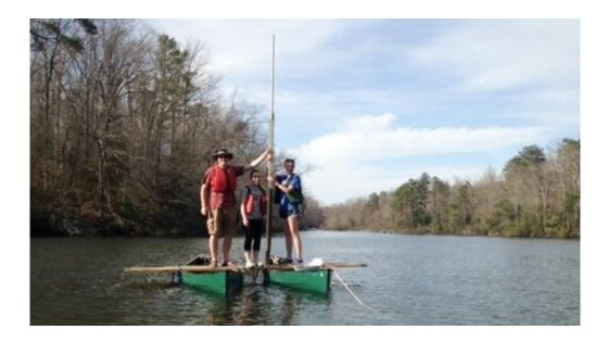
Red-shirted geologist Jim Kaste works with a couple of William & Mary undergraduates from a coring platform assembled from a couple of lashedtogether canoes on Lake Matoaka. Credit: W&M Dept. of Geology
