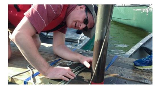
Geologist Jim Kaste inspects a sediment core fresh and dripping from the bottom of Lake Matoaka. The cores go back to the lab for sophisticated chemical analysis of particles that can be used to trace the progress of American industrial development. Credit: W&M Dept. of Geology
