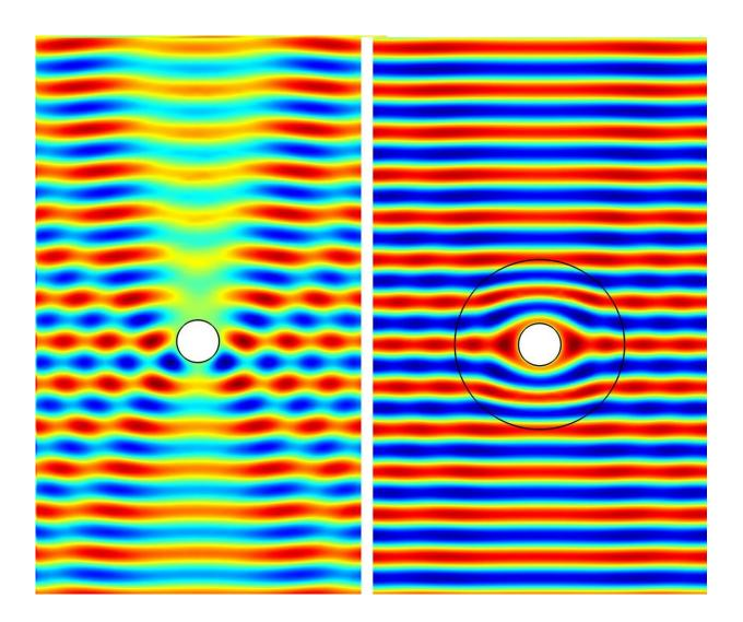
Invisibility cloaking illustrating how cloaking works using electromagnetic
