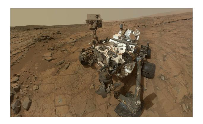
This self-portrait of NASA's Mars rover Curiosity combines dozens of exposures taken by the rover's Mars Hand Lens Imager (MAHLI) during the 177th Martian day, or sol, of Curiosity's work on Mars (Feb. 3, 2013), plus three exposures taken during Sol 270 (May 10, 2013) to update the appearance of part of the ground beside the rover. Credit: NASA
