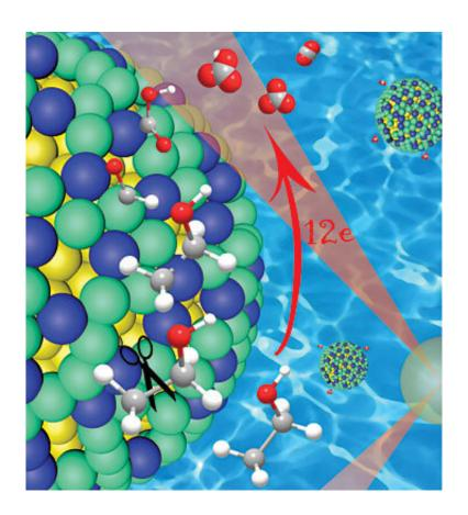
A close-up of the platinum/iridium (green/blue) shell over a gold nanoparticle core (yellow), showing how this catalyst cleaves the carbon-carbon (gray) bonds in ethanol while initially leaving hydrogen atoms attached. The hydrogen protects the carbon in the early stages of the reaction, preventing the formation of catalyst-poisoning carbon monoxide, which enables complete oxidation and the release of 12 electrons. Credit: Brookhaven National Laboratory
