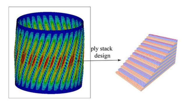
Simulation of buckling knockdown factor prediction for a composite shell (left), and the ply stack of the composite (right). Credit: Oak Ridge National Laboratory
