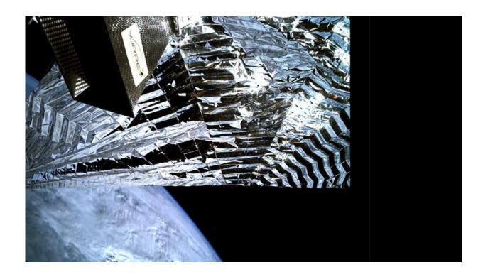
The Icarus-1 sail deployed on board TechDemoSat-1, with a view of Earth beyond. Credit: SSTL
