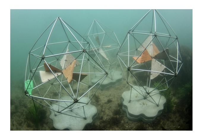
Created by Reef Design Lab, the metre-high pods are constructed from marinegrade steel and concrete and feature elements of 3D printed design. Half of the units have additional complexity in the form of triangular tiles. Data collected from the two different reef structures help inform future reef design. Credit: Alex Goad
