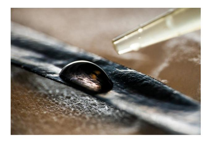
The artificial muscle developed by researchers at Linköping University consists of polymer material, into which the researchers have integrated enzymes. A solution of glucose and oxygen in water powers the polymer actuator, in a similar way as biological muscles. Credit: Thor Balkhed/Linköping University
