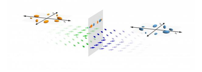
A domain wall (gray panel at center) separates regions with different spin orientations (green and blue arrows). MIT researchers discovered that a magnetic field applied at one particular angle through a single crystal of a new magnetic quantum material makes it harder for electrons to cross this domain wall. Credit: Leon Balents
