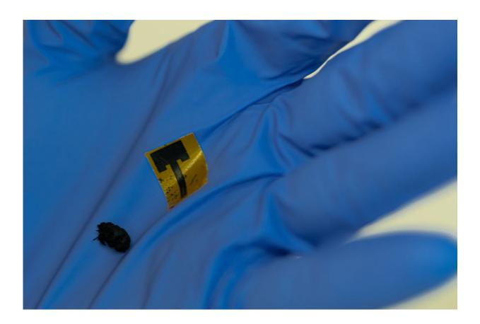
Metal-free antennas made of thin, strong, flexible carbon nanotube films are as efficient as common copper antennas, according to a new study by Rice University researchers. Credit: Jeff Fitlow
